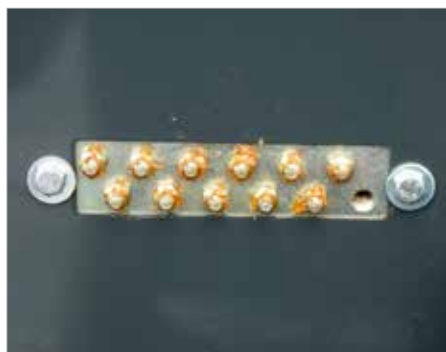
6. Centralised grease banks for roller bearings
