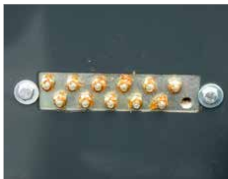
6. Centralised grease banks for roller bearings
