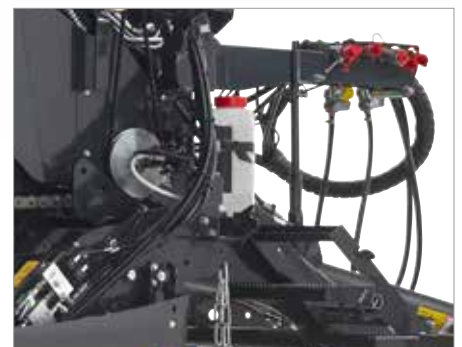
6. BEKA-MAX continuous chain oiling system
