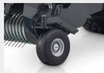
Pivoting semi-pneumatic pick-up guide wheels
