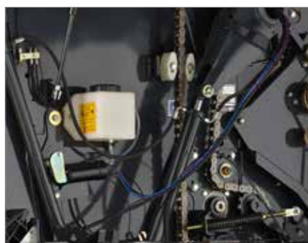
7. Automatic chain lubrication system
