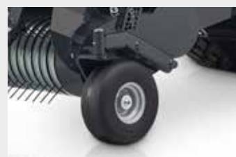
Pivoting semi-pneumatic pick-up guide wheels
