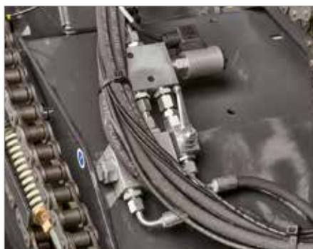
6. Separate knife / DROPFLOOR controlled from the tractor cab
