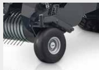
Pivoting semi-pneumatic pick-up guide wheels
