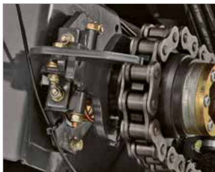
5. Mechanical rotor disengagement
