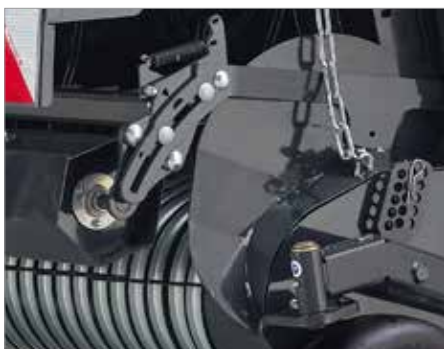
4. Spring-loaded crop tines and heavy crop roller (Ø 217 mm) for improved pre-compression and crop flow
