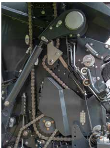
10. Robust driveline with wear-resistant and oversized chains
