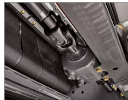
7. Heavy-duty cross joints in the drive axles
