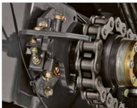
4. Mechanical rotor disengagement
