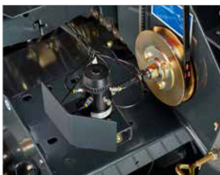
9. BEKA-MAX continuous chain lubrication system
